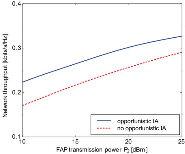
Fig. 8. Network throughput  $\mathcal{T}$  in bits/s/Hz as a function of the FAP transmission power  $P_2$  with and without opportunistic IA when  $\lambda = 1.59 \times 10^{-4}$  FAPs/m<sup>2</sup> and  $p = 0.2$ .
