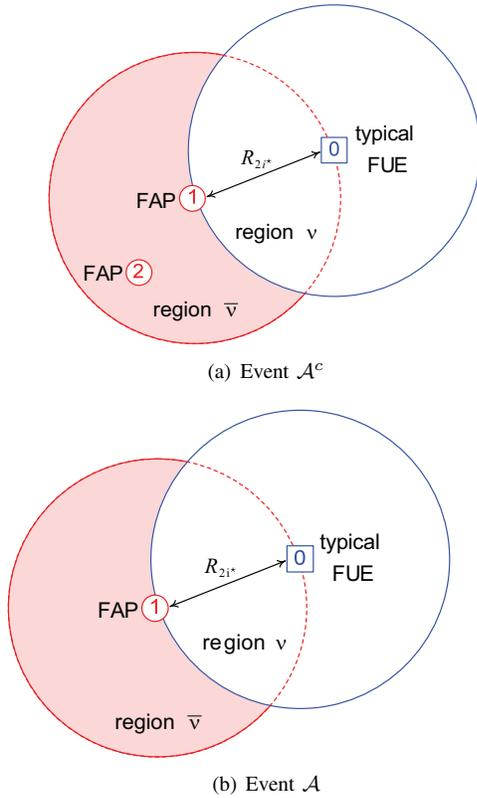
Fig. 1. Example scenarios where (a) the event  $\mathcal{A}$  that the typical FUE is capable of canceling its nearest interfering FAP  $i^*$  (i.e.,  $i^* = 1$ ) does not occur as there exist two FAPs (FAP 1 and FAP 2) in the region  $\bar{\mathcal{V}}(R_{2i^*})$ ; and (b) the event  $\mathcal{A}$  occurs as there is only one FAP in  $\bar{\mathcal{V}}(R_{2i^*})$ .
