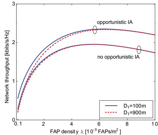
Fig. 7. Network throughput  $\mathcal{T}$  in bits/s/Hz as a function of the FAP density  $\lambda$  with and without opportunistic IA for  $p = 0.2$  when  $D_1 = 100$  and 900 meters.
