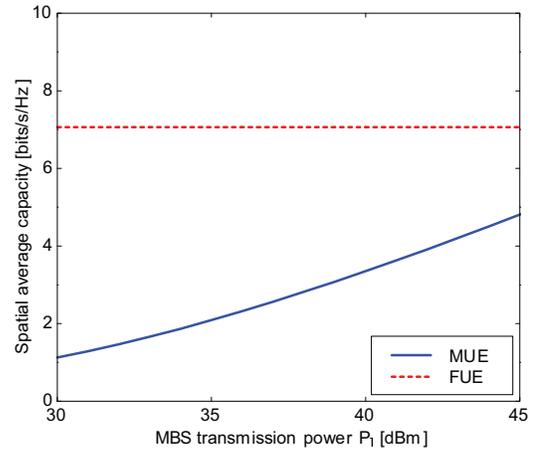
Fig. 6. Spatial average capacity in bits/s/Hz at the FUE and MUE for opportunistic IA as a function of the MBS transmission power  $P_1$  when  $\lambda = 1.59 \times 10^{-4}$  FAPs/m<sup>2</sup> and  $p = 0.2$ .
