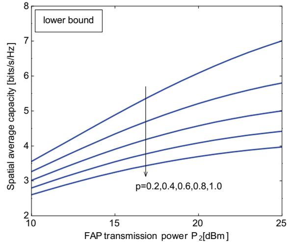
Fig. 10. Spatial average capacity in bits/s/Hz at the FUE as a function of the FAP transmission power  $P_2$  for opportunistic IA with imperfect CSI when  $p = 0.2, 0.4, 0.6, 0.8, 1.0$ , and  $\lambda = 1.59 \times 10^{-4}$  FAPs/m<sup>2</sup>.
