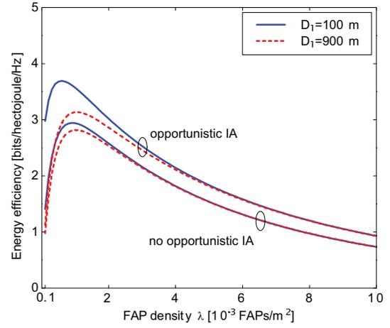
Fig. 9. Energy efficiency  $\mathcal{E}$  in bits/joule/Hz as a function of the FAP density  $\lambda$  with and without opportunistic IA for  $p = 0.2$  when  $D_1 = 100$  and 900 meters. In this example, we set  $Q_1 = 48.4$  dBm,  $Q_2 = 45.3$  dBm, and  $\beta_1 = \beta_2 = 5.5$ .
